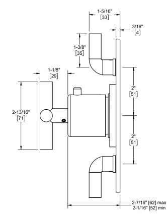
Dimensions are inches, rounded to 1/16" [Dimensions in brackets are mm, rounded to 1mm]
