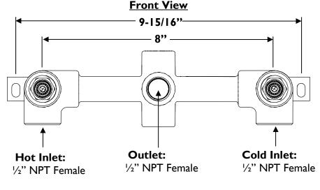
\*\*NOTE: Valve rough must be set back a minimum of 2-5/8" from finished wall surface to center of inlets
